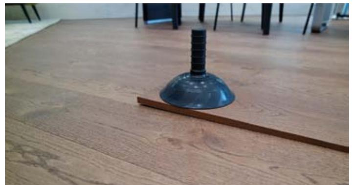
Using our recommended lifting device to remove Attiro.
